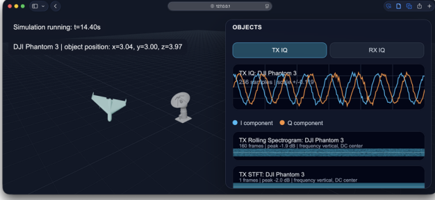
Fig. 2. The RF-UAVSim browser interface during a run: an analytic 3D scene (left) and live I/Q, rolling spectrogram, and current-window STFT (right). Displays are qualitative; all measurements use unrounded backend IQ.
