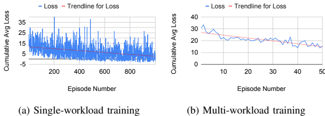
Fig. 5: Learning curve of FaaSRank through single-workload and multi-workload training
