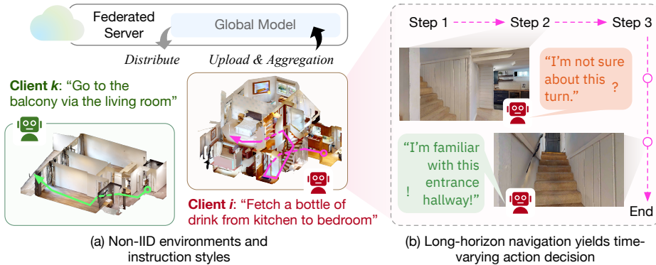
Fig. 1: Motivation of step-wise personalized federated VLN. (a) Client-induced heterogeneity: different houses exhibit distinct visual statistics, and users describe routes with diverse instruction styles, yielding severe non-IID data across clients in federated training. (b) Long-horizon, time-varying decision contexts: within a single episode, the agent may alternate between uncertain steps (e.g., unfamiliar turns) and confident steps (e.g., familiar hallways), motivating step-wise adaptation of personalization strength rather than a fixed per-client or per-episode strategy.
